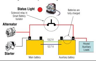
**2** When the engine is turned off, the alternator no longer supplies a charge to the batteries, and the loads on the batteries begin to deplete them.
