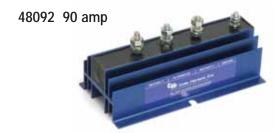
Terminations: three 1/4" (6.4mm) studs and one No. 10 stud. Two 9/32" (7.2mm) diameter mounting holes. Size: 6 1/2"L x 3 1/4"W x 2 13/16"H (165.0 x 82.6 x 71.0mm).
