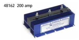
Terminations: three 5/16" (7.9mm) studs and one No.10 stud. Four 9/32" (7.2mm) diameter mounting holes. Size: 8 1/2"L x 4 3/16"W x 3 13/32"H (215.0 x 122.2 x 86.5mm).
