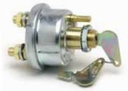
Mounting stem: Brass, 3/4" -16 thread 17/32" (13.5mm) long. Fits panels up to 1/4" (6.4mm) thick. Terminals: Two 3/8" -24 studs. Plated steel case, silver-laminated contacts. Hencol lock and 2 keys. Indexing pin.
