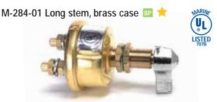
Mounting stem: Brass 3/4" -16 thread (19.1mm), 1 13/32" (46.1mm) long. Fits panels up to 15/16" (23.8mm) thick. Terminals: Two 3/8" (9.5mm) diameter studs. Actuator: Chromeplated lever. Silver-laminated contacts. Labeled UL 707B.
