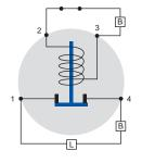
Solenoid in its normal state Control circut and load circuit open
