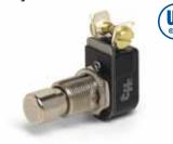
6A at 125V, 3A at 250V. Push On, spring return to Off. For AC or DC. UL-approved. Plastic body, nickel-plated plunger. Two screw terminals. 15/32" –32 mounting stem, 9/16" (14.3mm) long.
