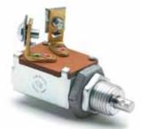
10A at 12V DC. Normally Off. Pull On, spring return to Off. Brass case and mounting hardware. Two screw terminals with lockwashers. Mounting stem 1/2"-20 thread, 5/8"(15.9mm) long. No knob: shaft has 3/32" (2.4mm) hole for the attachment of a cable or lever.
