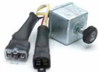
Controls two motors. One Delphi (Packard) 4-way male connector 6294544 (mates with 2977048) and one Delphi (Packard) 6-way male connector 2977042 (mates with 2977044). With round knob imprinted with SAE washer-wiper symbol. Lead and connector assembly: 5.625" (142.9mm) long.
