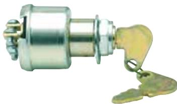
Three screw terminals. Plated steel case. 5/8" -32 mounting stem, fits panels up to 9/16" (14.3mm). With O-ring seal.
