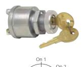
Key removable in both positions. Electrical ratings at 12V DC: 10A both positions. Three brass screw terminals. Diecast case. Mounting stem 3/4" -20, 13/16" (20.6mm) long, fits panels up to 1/4" (6.4mm). Knurled aluminum adapter facenut permits mounting in 3/4" (19.1mm) to 7/8" (22.2mm) diameter holes.
