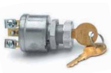
Three screw terminals. Zinc diecast case. 3/4" -20 mounting stem, fits panels up to 11/64" (4.4mm).
