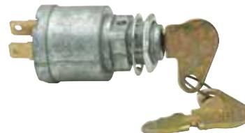
Electrical ratings at 12V DC: 5A Start, 1A Magneto. Three blade terminals. Diecast zinc case. 5/8" -32 mounting stem with O-ring seal, fits panels up to 7/32" (5.5mm). Mates with Delphi (Packard) connector 2973422.
