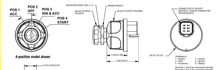
**Battery Start** Accessory Ignition Terminals 1 & 6 **Terminal 2** Terminal 3 Terminals 4 & 5 **Position 1 Position 2** Х **Position 3** Х Х Χ **Position 4**
