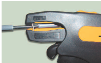
1. Slide the adjustment to the appropriate wire type
