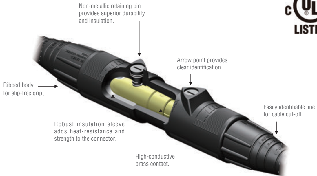
Wide range cable access form 0.33" to 1"
