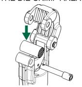
3. CLOSE THE TOP OF THE TOOL HEAD AND INSERT PIN STOP
