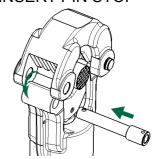
4. USE THE HANDLE TO ADVANCE THE CRIMP HEAD UNTIL IT CONTACTS THE TERMINAL. CHECK TERMINAL ALIGNMENT WITH CRIMP HEAD. COMPLETE CRIMP BY ADVANCING CRIMP HEAD WITH HANDLE.
