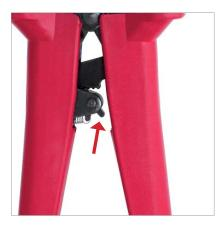
Push the release lever of the ratchet upwards. Tool opens automatically.
