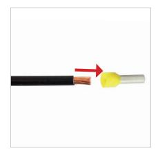
2 Strip the wire to the correct length and insert it into the terminal until stop.
