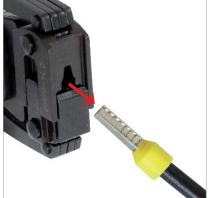
4 Remove correct crimped terminal out of the tool.
