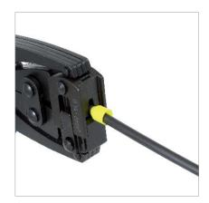
3 Insert precisely stripped wire with the wire end ferrule into the profile. Close the tool until it opens automatically.
