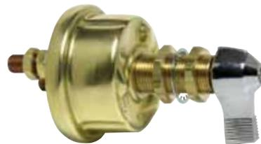
Brass case. Silver laminated contacts. Chrome-plated diecast lever. Brass mounting stem 3/4" -16 thread 1 13/32" (46.1mm) long. Fits panels through 15/16" (23.8mm) thick. Two 3/8" -24 and two 10-32 studs. Labeled UL 707B.
