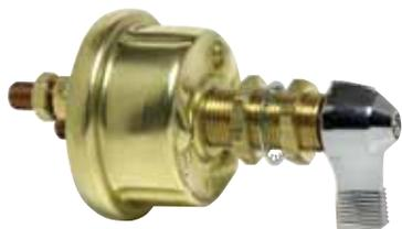
Chrome-plated diecast lever. Brass mounting stem 3/4" -16 thread 1 13/32" (46.1mm) long. Fits panels through 15/16" (23.8mm) thick. Two 3/8" -24 and two 10-32 studs.
