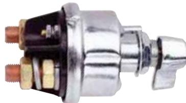
Electrical ratings: Large studs: 2000A intermittent, 30 seconds On, 3 minutes Off. 300A continuous. Small studs: 20A continuous. Plated steel case. Chrome-plated diecast lever. Mounting stem 3/4" -16 thread, fits panels through 1/4" (6.4mm) thick. Two 1/2" -20 copper and two 10-32 studs. Sealed between shaft and mounting stem, and case and terminal insulator. With indexing pin.
